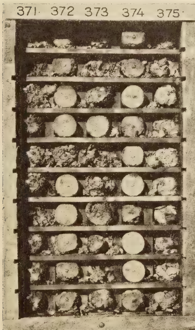
FIGURE 8.—VARIOUS COMPARISONS SHOWING FAVORABLE RESULTS OBTAINED WITH HIGH ALUMINA CEMENTS
